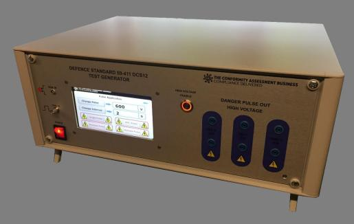
The Conformity Assessment Business Model DCS12 Test Generator meets all the DCS12 wave verification parameters for testing DC, single and three phase equipment, that is source impedance and verification of damping and frequency when measured into a 10  $\Omega$  load. Output amplitude is software adjustable with permanent memory, should re-alignment be needed during calibration.
